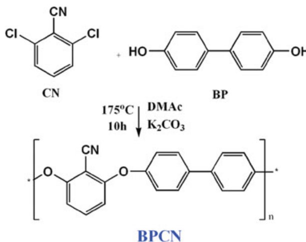
Figure 1 Synthesis of BPCN. [Color figure can be viewed in the online issue, which is available at www.interscience.wiley.com .]
